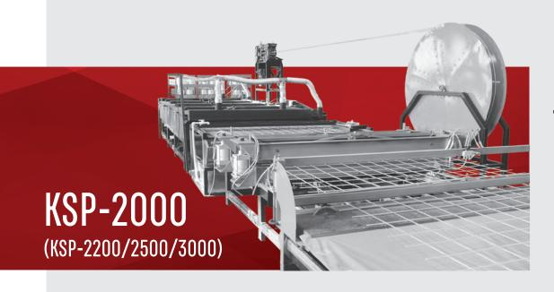
PRODUCTION LINE FOR THE MANUFACTURING OF FIBERGLASS MASONRY MESH WITH A BAR DIAMETER OF 2 TO 12 MM
